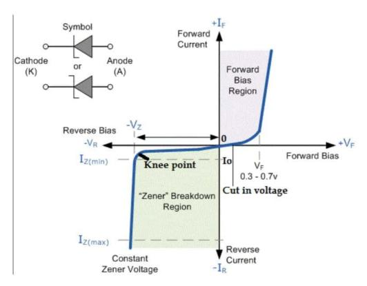
The above diagram shows the V-I characteristics of a zener diode. When the diode is connected in forward bias, this diode acts as a normal diode but when the reverse bias voltage is greater than zener voltage, a sharp breakdown takes place. In the V-I characteristics above  $V_z$  is the zener voltage. It is also the knee voltage because at this point the current increases very rapidly.
