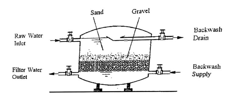
Closed rapid sand filter (pressure filter).
