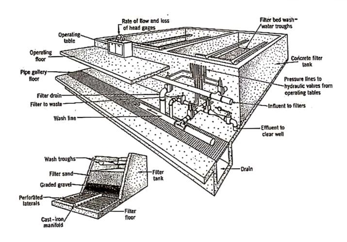
Components of an open (gravity) rapid
