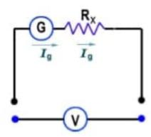
If potential between the points to be measured = V and if galvanometer gives fullscale deflection, when current "Ig" passes through it. Then,
